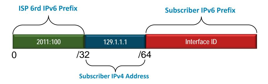
/64 does not work with multiple subnets Breaks existing residential IPv6 equipment Does not allow IP routing, forces bridging Leads to IPv6 NAT
