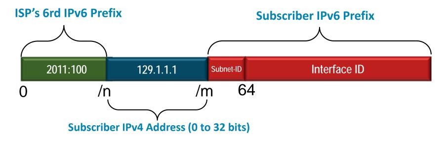
The construction is what allows 6rd to be stateless and SP-managed
